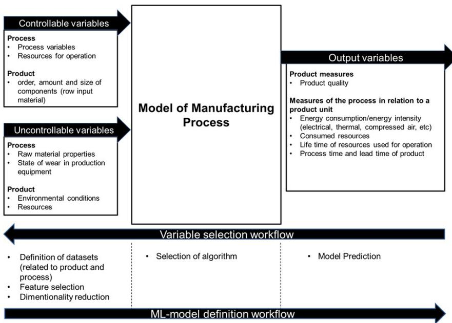
Figure 4. General data-driven modelling approach for manufacturing processes.
