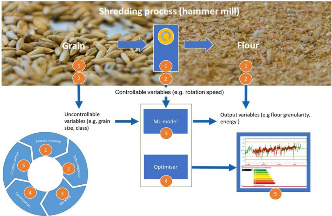
Figure 5. Overview of use-case in feed production.
