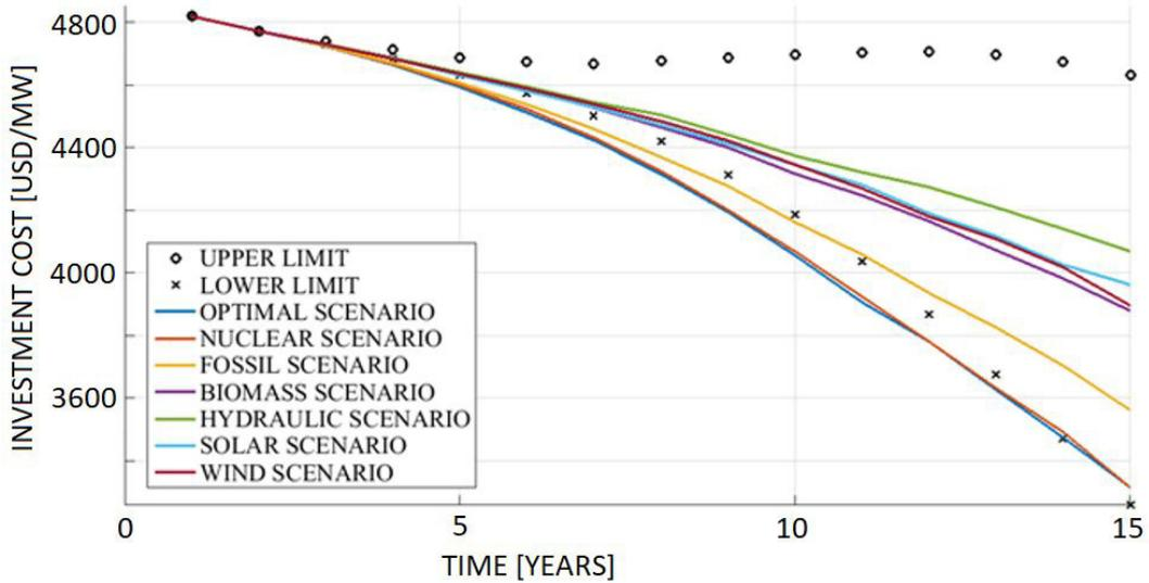
Figure 6. Investment Cost [USD/MW] vs. time in years, for the Optimal Scenario. Source: The Author.
