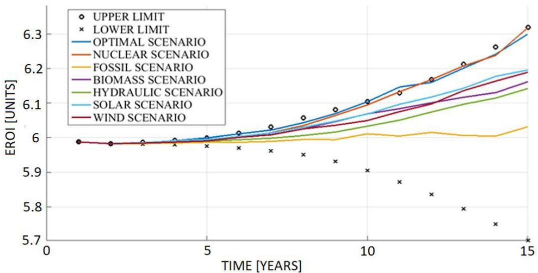
Figure 4. Energy Returned On Investment (EROI) vs. time [years] for the Optimal Scenario. Source: The Authors.
