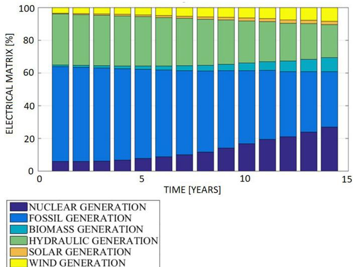
Figure 3. Electrical matrix (%) vs. time in years for the Optimal Scenario. Source: The author.
