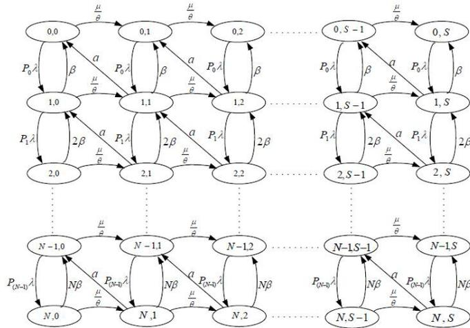
Figure 4. First scenario state transition rates diagram.
