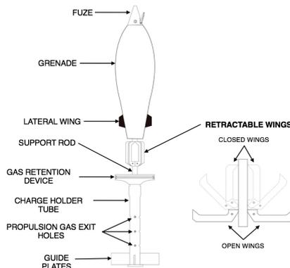
Figure 8. External view of mortar ammunition concept.
