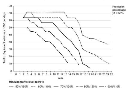
Figure 5. Traffic threshold curves (with min/max traffic level options and 50% protection).
