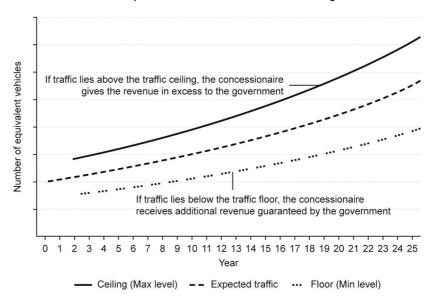
Figure 1. Project with one floor and one ceiling.
